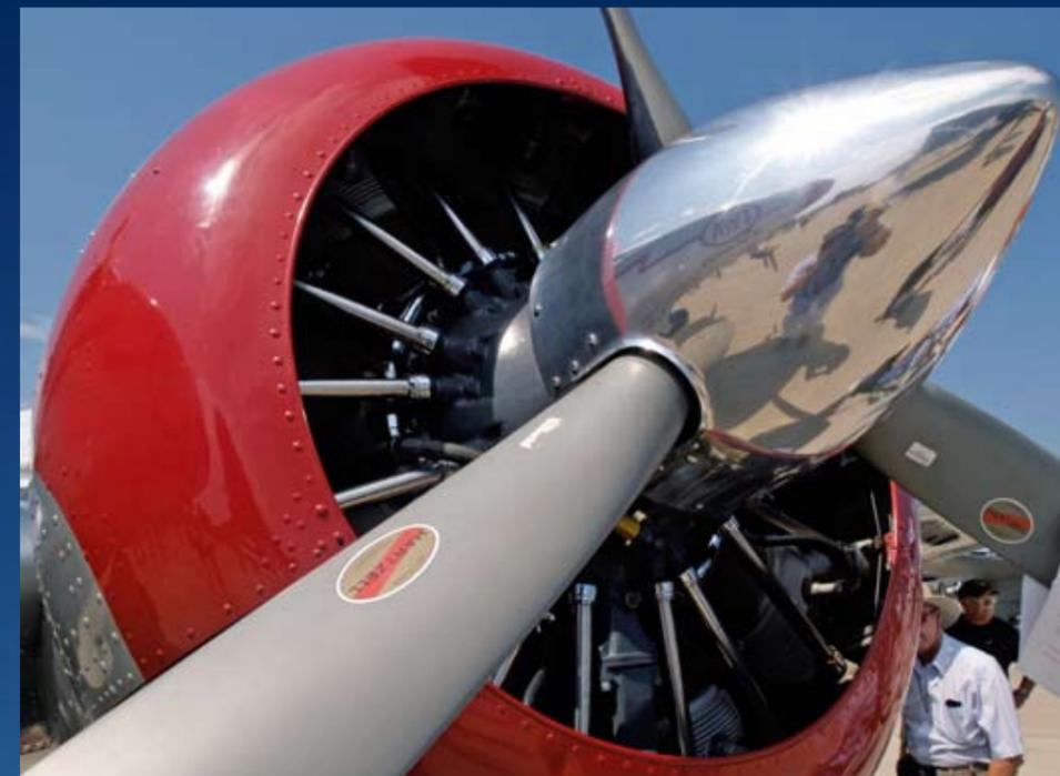
**ABOVE** The two large 450hp Pratt & Whitney R-985 radial engines are not the most economical of powerplants and typically they burn between 165 and 190lbs of fuel per hour... each!
